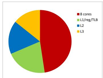
Figure 1.1.7: Power breakdown of an 8 core server chip.
