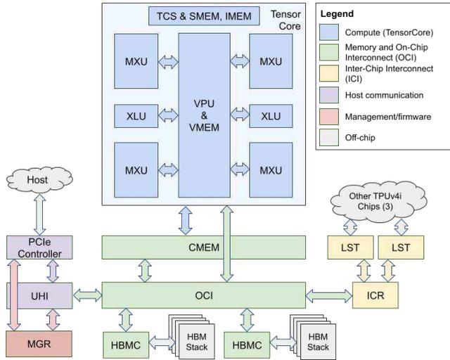
**Figure 5. TPUv4i chip block diagram.** Architectural memories are HBM, Common Memory (CMEM), Vector Memory (VMEM), Scalar Memory (SMEM), and Instruction Memory (IMEM). The data path is the Matrix Multiply Unit (MXU), Vector Processing Unit (VPU), Cross-Lane Unit (XLU), and TensorCore Sequencer (TCS). The uncore (everything not in blue) includes the On-Chip Interconnect (OCI), ICI Router (ICR), ICI Link Stack (LST), HBM Controller (HBMC), Unified Host Interface (UHI), and Chip Manager (MGR).
