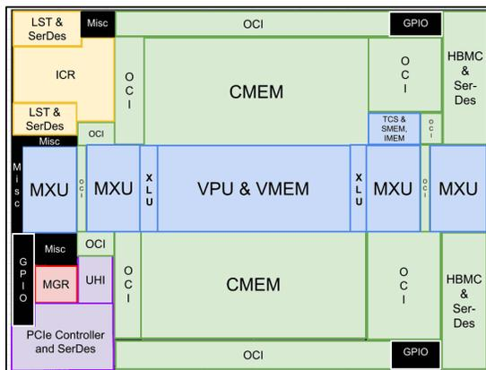
**Figure 6. TPUv4i chip floorplan.** The die is <math><400 \text{ mm}^2</math> (see Table 1). CMEM is 28% of the area. OCI blocks are stretched to fill space in the abutted floorplan because the die dimensions and overall layout are dominated by the TensorCore, CMEM, and SerDes locations. The TensorCore and CMEM block arrangements are derived from the TPUv4 floorplan.
