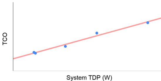
**Figure 3. TCO vs system TDP for T4 and TPUv1/v2/v3/v4i. An  $R^2$  of 0.982 means  $R$  is nearly perfect at 0.99 out of 1.00. System TDP is capacity planning power and not average power, since capacity is more expensive (see §7.D for details).**
