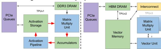
**Figure 1. TPUv1 block diagram (left) vs TPUv2/v3.**
